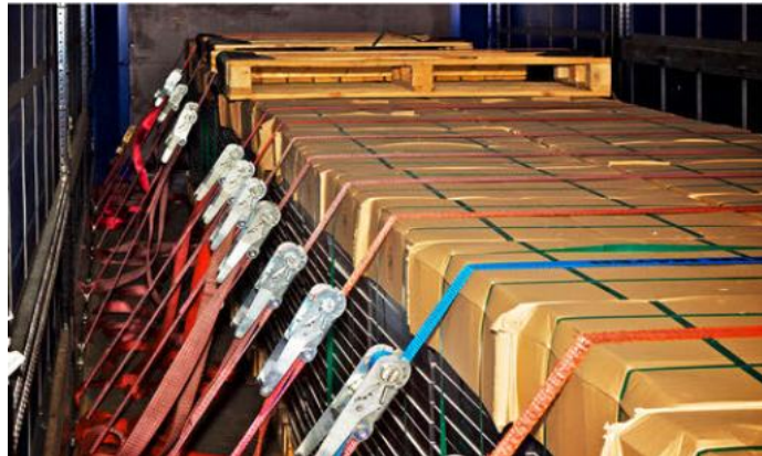
Cargo Lashing With Egro Ratchet European Type EN-12195-2
